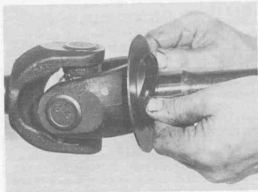
Figure 71 1019-71 Assemble new seal as shown. Lip of the seal is to be directed towards the spindle.
