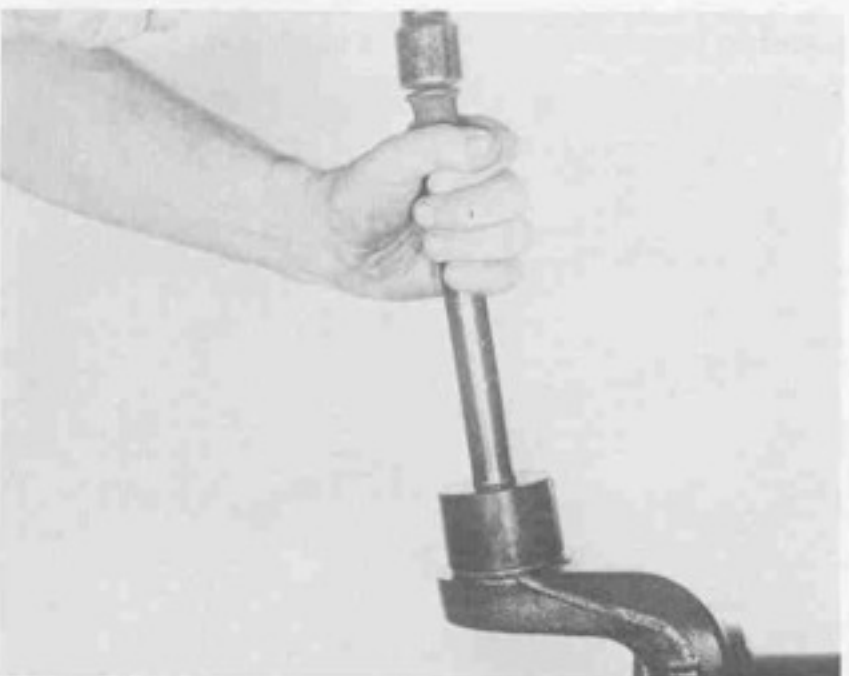
Figure 63 1019-63 Fill the area in grease retainer with specified grease, grease bearing cone and install. Install new king pin bearing oil seal.
