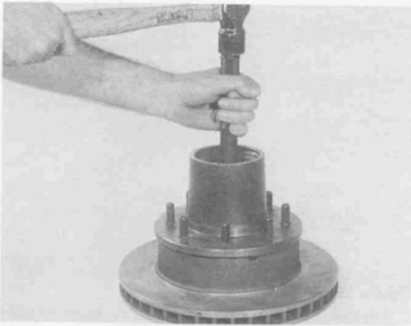
Figure 49 1019-49 Assemble outer wheel bearing cup. Tools: #D-254 Installer, #C-4171 Handle.
