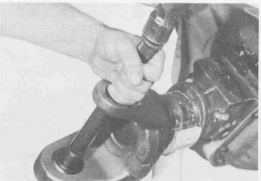
Figure 61 1019-61 Remove king pin bearing cup, cone, grease retainer, and seal all at the same time. Assemble and use tools exactly as shown in Figure 62. Discard seal and replace with new one at time of assembly. If grease retainer is damaged, replace with new one at time of assembly.
