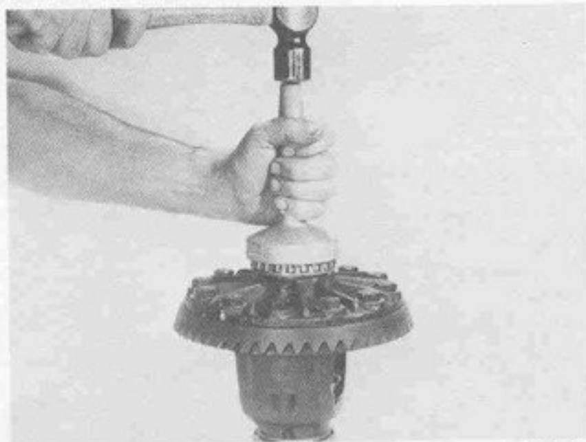
Figure 187 1019-187 Assemble the required amount of shim onto hub (ring gear side) as determined in figure 186. Place bearing cone on hub of case. Use bearing installer to seat bearing cone as shown.
