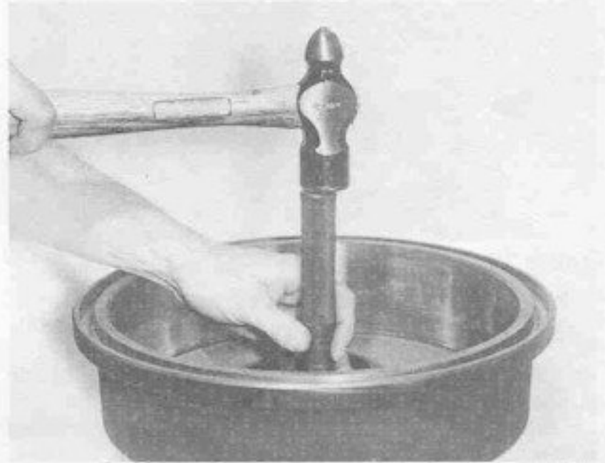
Figure 12 1019-12 Remove inner and outer wheel bearing cups. Tools: #D-255 Cup Remover, #C-4171 Handle.
