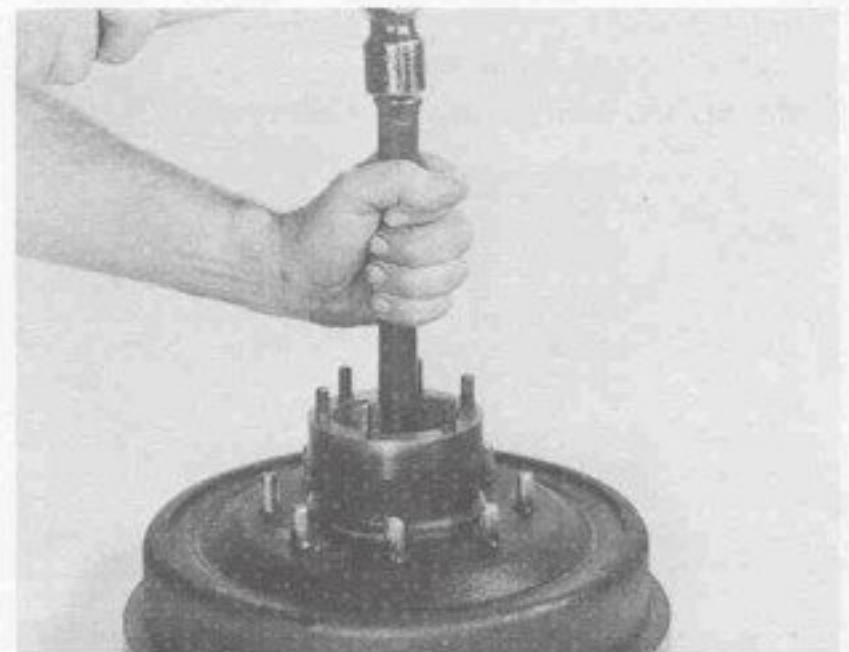
Figure 13 1019-13 Assemble outer wheel bearing cup. Tools: #C-4023 Installer, #C-4171 Handle.
