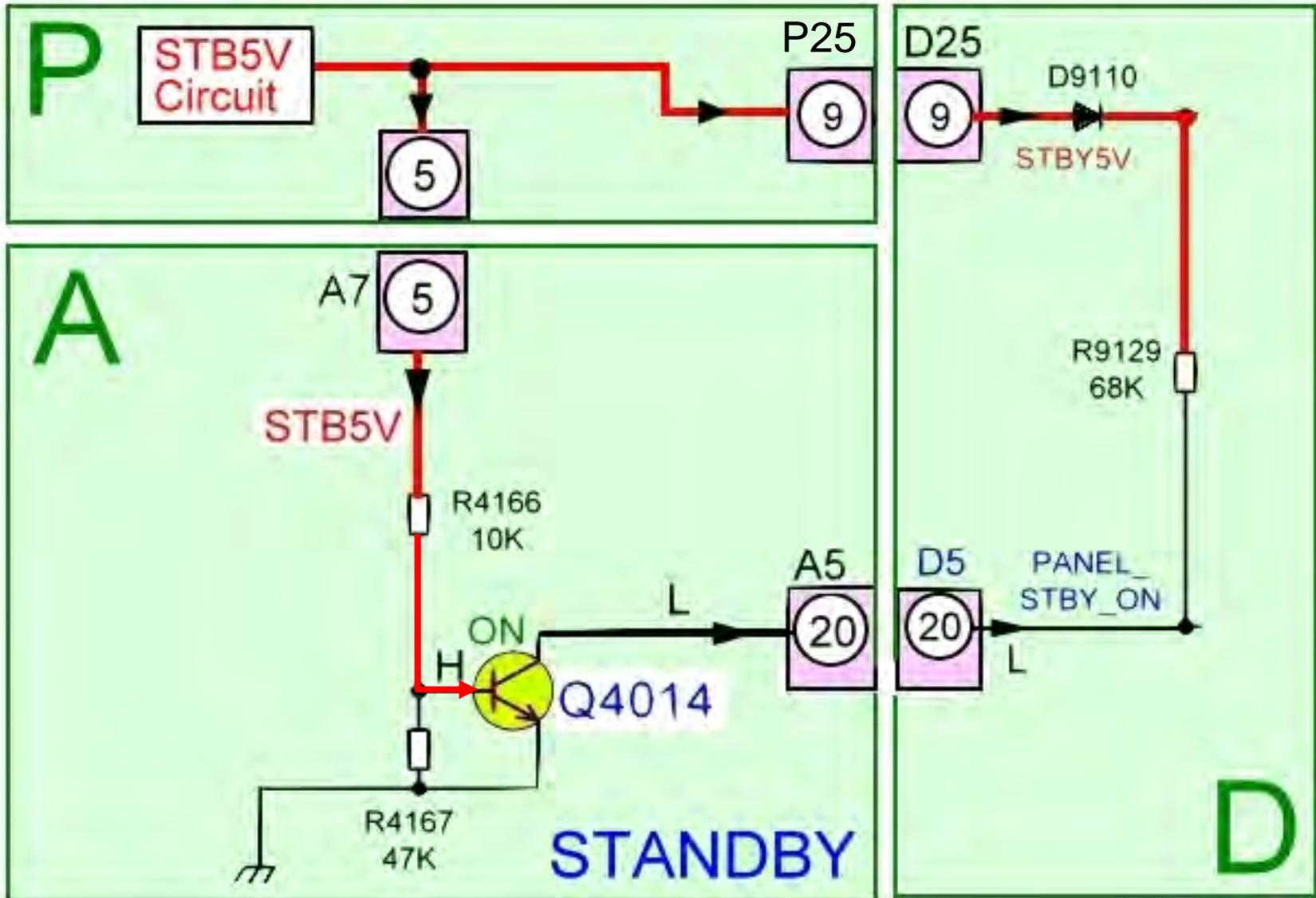
This circuit combined with the circuit in the following page is used to explain the reason why the CPU (IC9003) on the D board is not active during Standby. The transistor Q9014 is on to keep PANEL\_STBY\_ON low.
