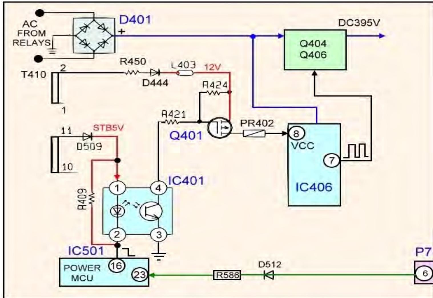
Pin 16 of IC501 also goes low when pin 23 is “high”. When pin 16 goes “low”, the diode within the photo-coupler IC401 emits light to turn on the photo-transistor.
