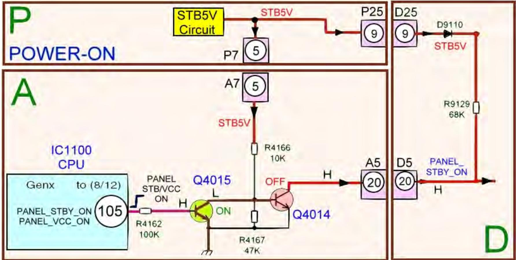
Upon receiving the power on command , the “PANEL STB/VCC ON” pin of the main MPU (IC1100) outputs 2.5V to the base of Q4015, turning it on. Q4015 outputs a low to turn off Q4014 allowing pin 20 of the connector A5/D5 to go high.
