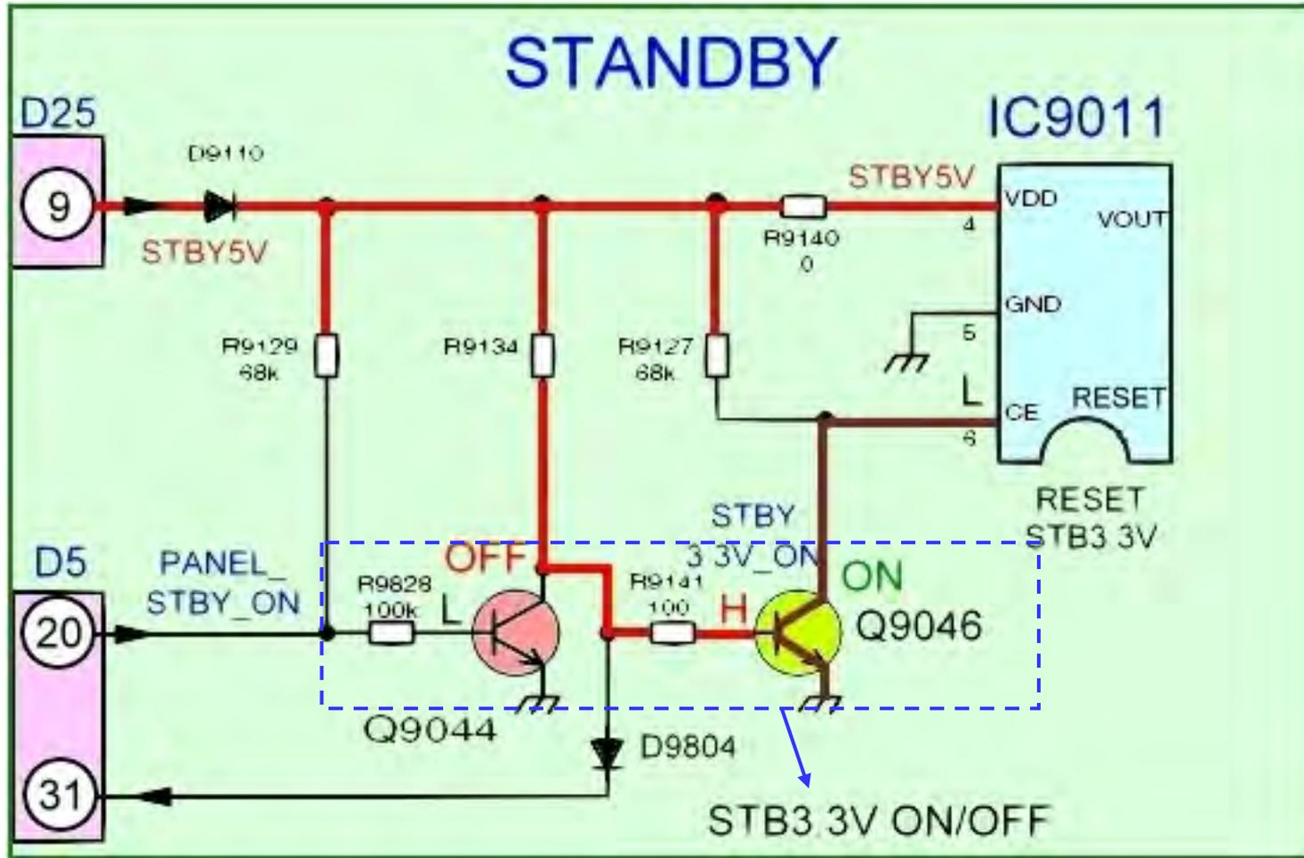
The STB5V source is connected to the voltage input (pin 4) of the RESET/STB3.3V regulator IC9011. The output of this IC is controlled by the ON/OFF pin (Pin 6). The DC level of this pin is determined by the "STB3.3V ON/OFF" circuit.
