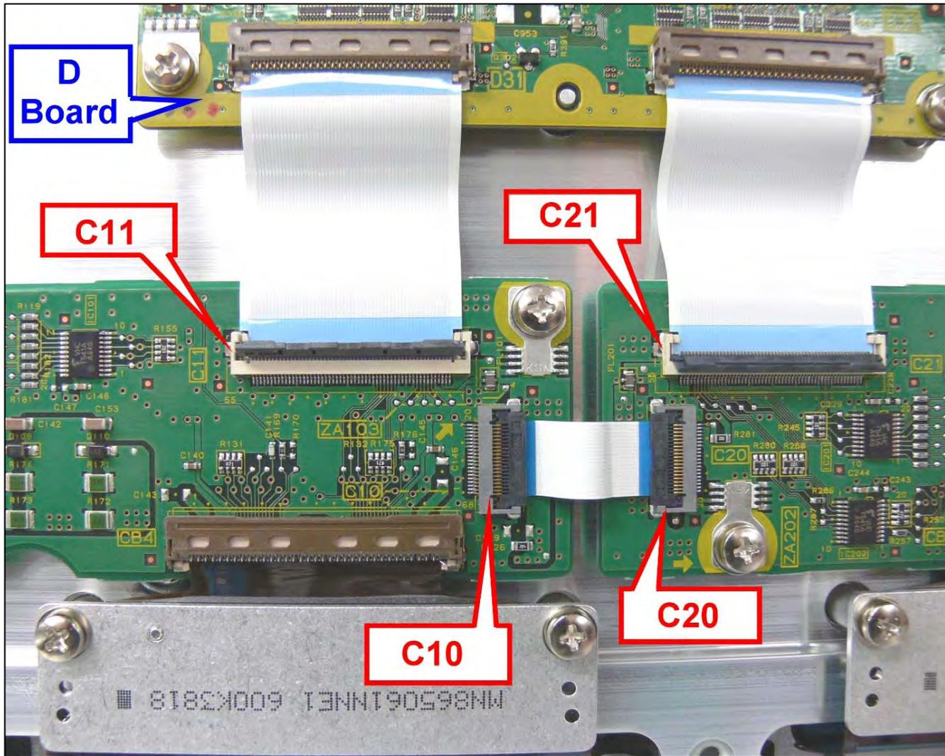
The improper connection of the connectors D31/C11, D32/C21, C10 and C20 causes a DVR\_RST SOS. The power LED blinks 6 times, leading one to believe that there is a problem in the scan output circuit.
