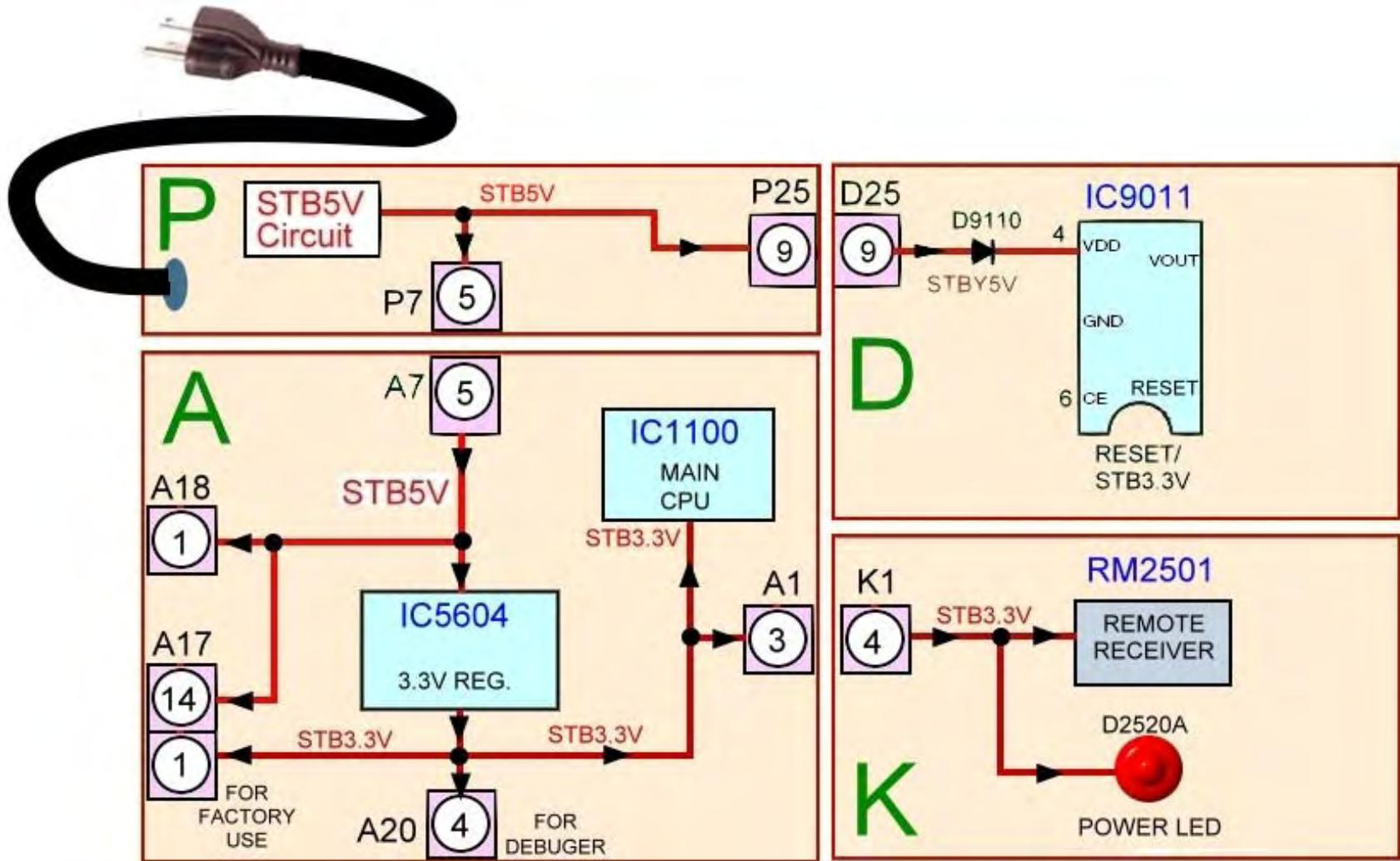
The STB5V is connected to the D and A boards. During standby, this voltage is not used by the D board. On the A board, the STB5V is applied to a 3.3V regulator (IC5604) to generate the STB3.3V to power the MAIN MICON Genx4 (IC1100). The STB3.3V is also connected to the remote receiver IC and the power LED on the K board.
