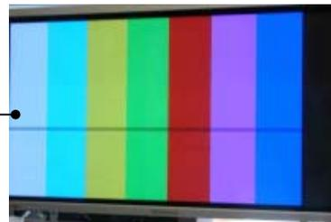
In case of horizontal line problem, first, check the connection of FPC between SU/SD board and the panel.
