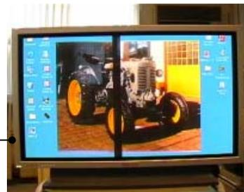
In case of vertical picture problem, first, check the connection of FPC between A board and C board.
